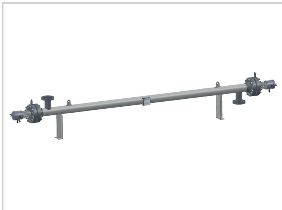
Electric heat exchangers to heat liquid or aeriform fluids with varying pressure up to 300 bar. Used in cases of high differences in inlet and outlet temperature and in cases of installations requiring a high energy input. Designed with a single vessel on which a heater is installed on either side. The reason for a dual head is to limit the temperature on the surface of the heaters as a consequence of a wide range of variation of process temperatures.
