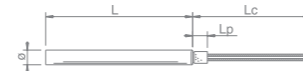
Type S with ceramic isolator Cartridge heater with internal connections with a ceramic insulator. The ceramic insulator (Lp in the figure) footprint is a maximum of 10 mm.
