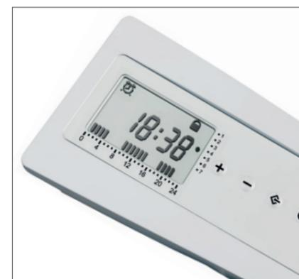
ON/OFF button changes the operating mode, sets the bar of the weekly program graph and the room temperature. The operating modes are: room temperature level (regulates the temperature not considering the timer program), timer, anti-freeze (energize the heater when room temperature is below 7°C), boost function and Fil-Pilote (via black dedicated wire).
