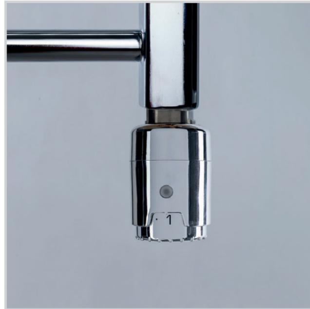
MOEBIUS is an electromechanical thermostatic water temperature heating system for towel rails filled with water, water and glycol or diathermic oil. The thermostatic control is fixed to a PTC Class I heating element and have a cable. The heating system can be installed in a stand alone towel rail or a towel rails connected to the central heating system. Water temperature regulation range from 5°C to 70°C.
